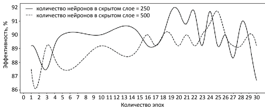
Fig. 5. Dependence of efficiency on the number of epochs when processing a Google set
