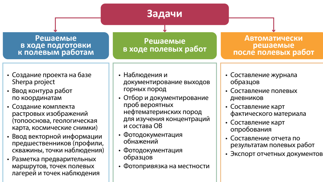
Fig. 3. Tasks solved with the help of the Sherpa software package during the field work of the FSBI VNIGNI, 2023
