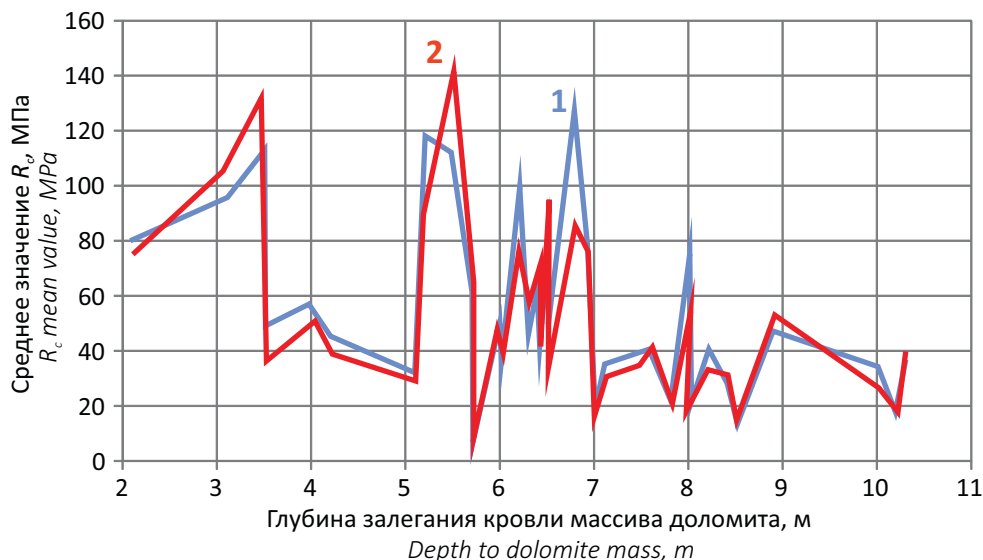
Fig. 6. Variation in average dolomite strength along the Amur-Yakutsk Railway route centerline derived
